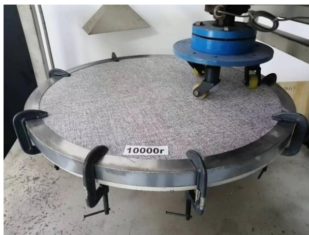
Fig 2. After test 10000r
