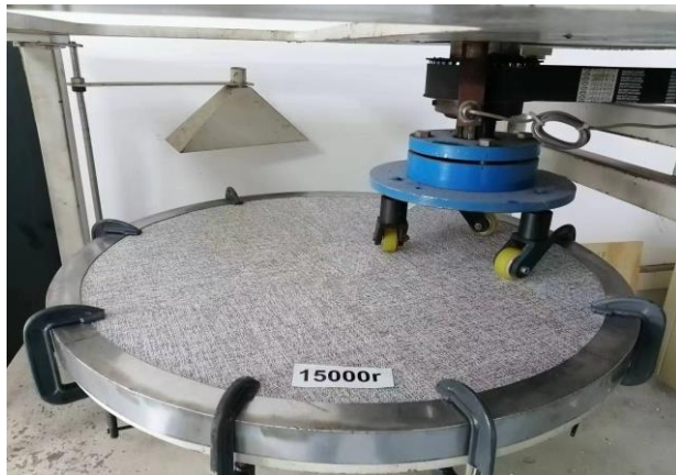
Fig 3. After test 15000r
