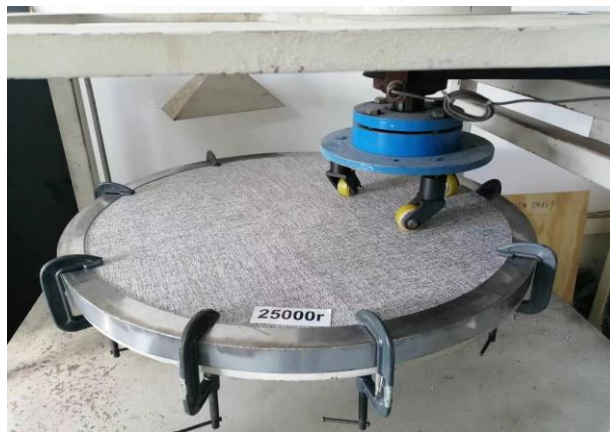
Fig 5. After test 25000r
